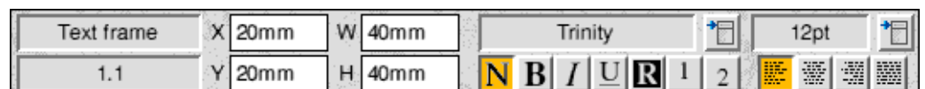
Fig. 8.26 - The info palette gives the size of the selected object. You can resize it by changing the W and H values and move it by changing the X and Y values.
